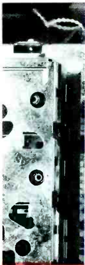
Top row terminals on the 9-87 module (left in picture) start with U14 at the left edge by even numbers to W15 at the right. Bottom terminals go from W1 at the left edge by odd numbers to U14 at the right. Top row of terminals on the 9-88 module (at right) starts with W15 at the left edge and go by odd numbers to W1 at the right. At the bottom terminals go from U14 at the left by even numbers to U2 at the right.
