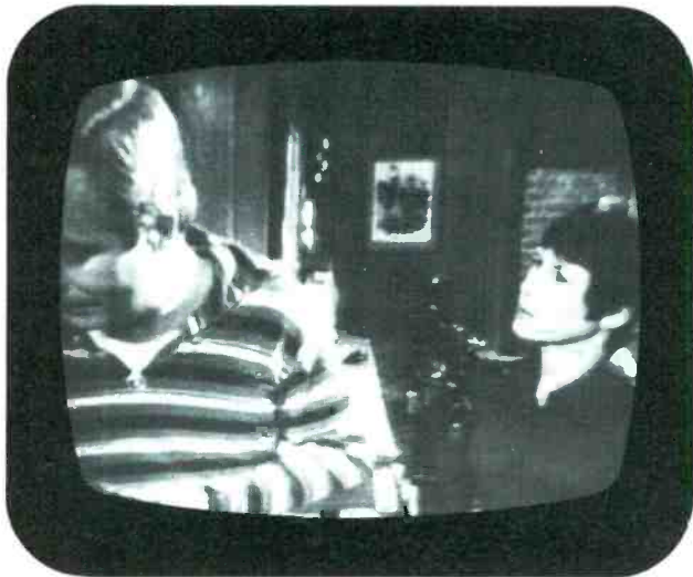
16 —Excessive contrast can result from misadjusted AGC and contrast controls, or perhaps from a borderline defect in the AGC circuit. The composite video is negative-going; therefore, too much video causes a darker picture.
