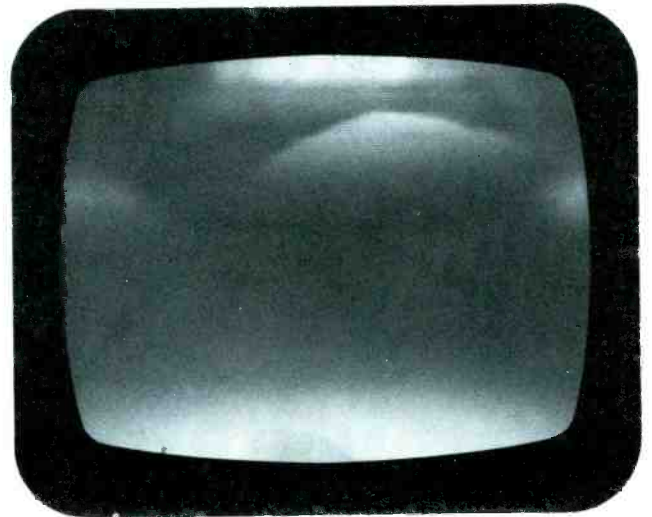
7—One light or dark large hum bar with rounded edges moving slowly up the picture usually is caused by a sine-wave 60-Hz voltage getting into video or chroma circuits, possibly by heater-to-cathode leakage in a tube. If the bar is not so wide (tall), it might be caused by insufficient filtering of the DC voltage from a power supply that does not double the ripple frequency.
