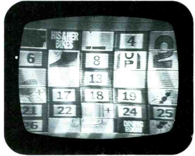
15—Interference that is not phase locked to the sweep frequencies (such as radiated noise from HV arcs, etc.) often appears in a Figure "S" shape. Most such lines are narrow; these were made wide by using a carrier modulated by square waves.
